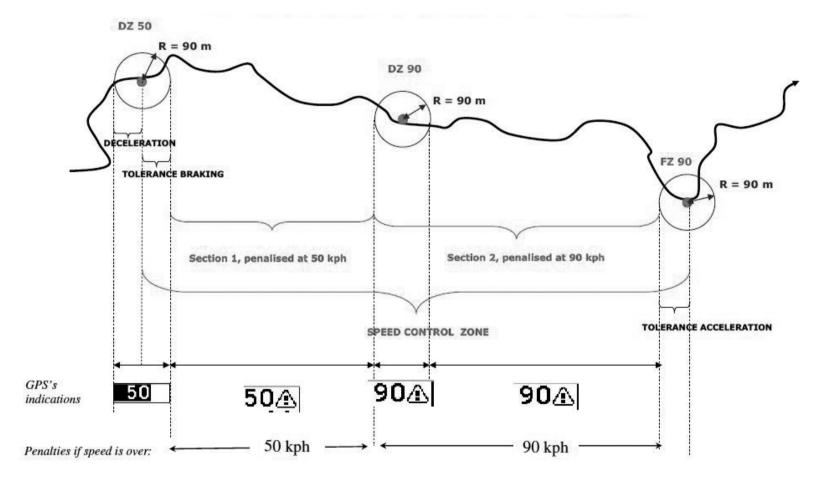
2 SUCCESSIVE SECTIONS, INCREASING SPEEDS: 50 TO 90 KM/H
